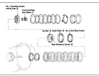
One-way clutch No. 1 (F1) operates with the second brake (B2) prevent the sun gear from turning counterclockwise. The one-way clutch No. 2 (F2) prevents the rear planetary carrier from turning counterclockwise.
