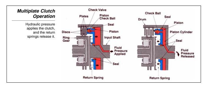
Hydraulic pressure actuates the piston and return springs return the piston to the rest position in the clutch drum when pressure is released. Friction discs are steel plates to which friction material is bonded. They are always located between two steel plates. The friction disc inner diameter is slotted to fit over the splines of the clutch hub.
