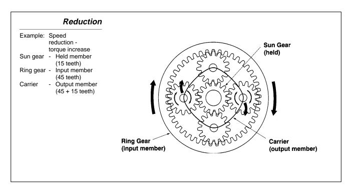
The gear ratio is computed as follows:
