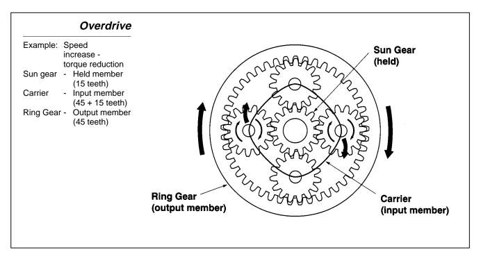
The gear ratio is computed as follows:
