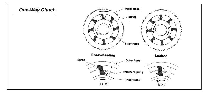
When the center race turns counterclockwise, it tries to move the sprag so that the long distance is wedged against the outer race. This causes the center race to stop turning. To assist the sprags in their wedging action, a retainer spring is installed, which keeps the sprags slightly tilted at all times in the direction which will lock the turning race.
