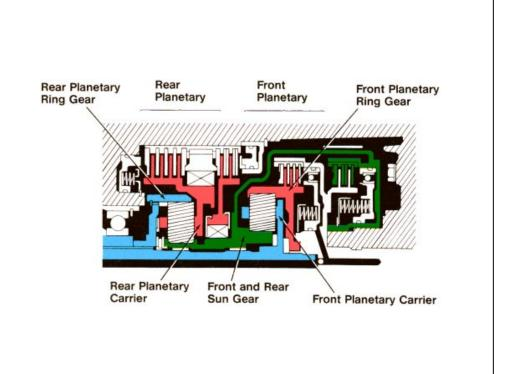
These planetary gear sets, the brakes and clutches that control their rotation, and the bearings and shafts for torque transmission are called the planetary gear unit.
