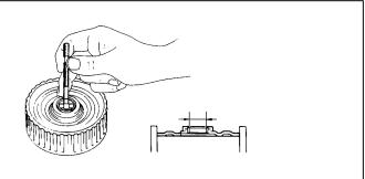
Use a feeler gauge to measure the clearance of the pinion gear to carrier housing and compare to the specifications. Standard clearance is 0.0079" to 0.0197". Clearance in excess of the standard on any planetary gear would require the replacement of the carrier assembly.
